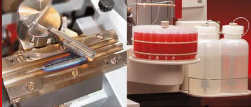
▲ Scraper – automatic cleaning module
